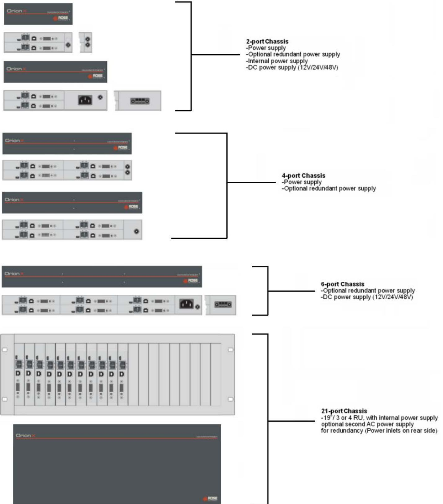
Figure 6. Orion Xtender Chassis Models
