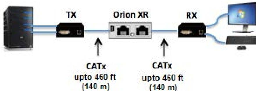
Figure 2. A Single CATx/CATx Repeater Doubles Extension Distance
