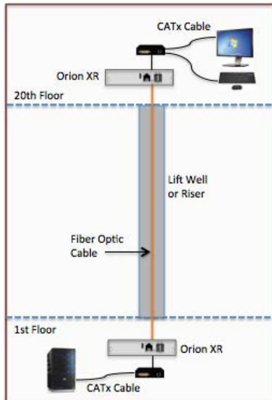
Figure 1. Cross-conversion of CATx and Fiber Signals Allow Extension to Great Distances
