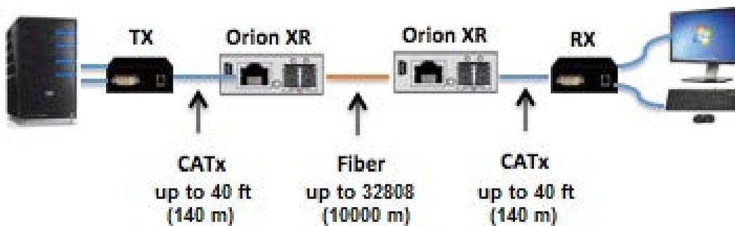
Figure 3. Two CATx/Fiber Repeaters Allow Extension to Greater Distances
