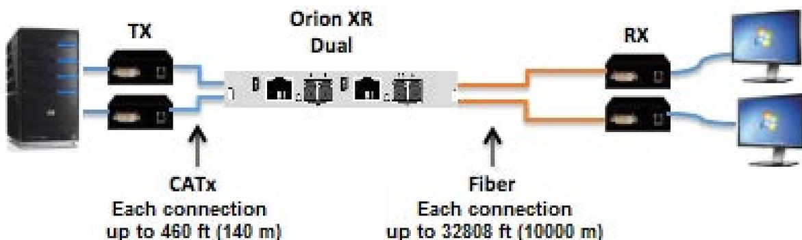
Figure 4. Dual CATx/Fiber Repeater Allows One Unit to Connect Two Sets of Extenders
